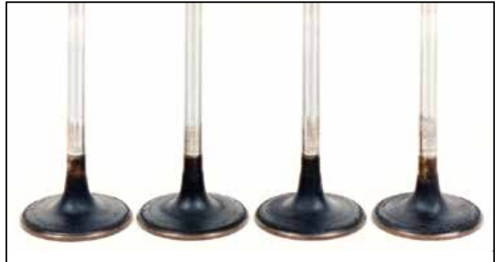
After 5,000 miles (8,000 km), an untreated reference gasoline left deposits on each intake valve.
